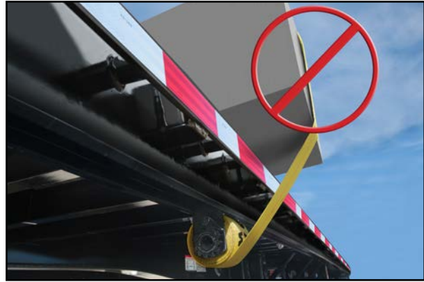
Figure 3: Double Wrap Strap Hook Secured on Side Rail WLL = 5400 lbs. (2449 kgs)
