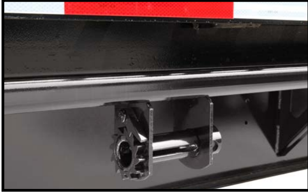
Figure 1: Sliding Winch in Integral Track on Siderail WLL = 5400 lbs. (2449 kgs)
