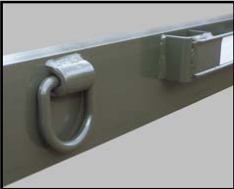
Figure – 14 “LASHING RING” Side Rail Mount WLL = 5400 lbs ( 2449 kgs)
