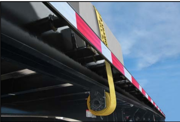
Figure 2: Single Wrap Strap Hook Secured on Side Rail WLL = 5400 lbs. (2449 kgs)
