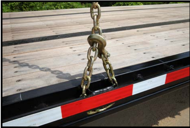
Figure 1: Chain securement around stake pocket WLL = 5400 lbs. (2449 kgs)
