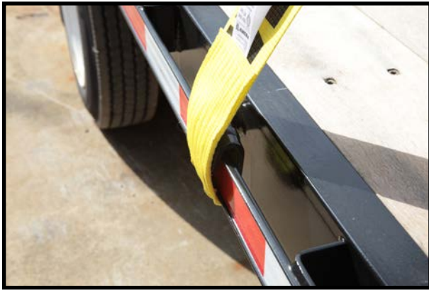
Figure 2: Single Wrap Strap Hook Secured on Side Rail WLL = 5400 lbs. (2449 kgs)
