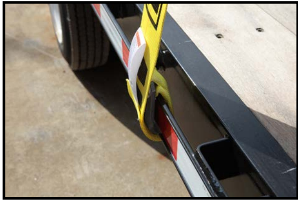
Figure 3: Double Wrap Strap Hook Secured on Side Rail WLL = 5400 lbs. (2449 kgs)
