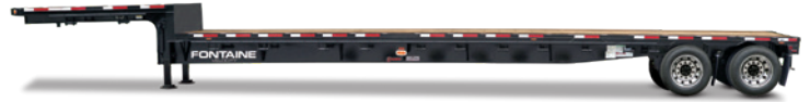
Velocity closed spring or air ride tandem dropdeck 48' configuration • Frame rating 80,000 lbs distributed
