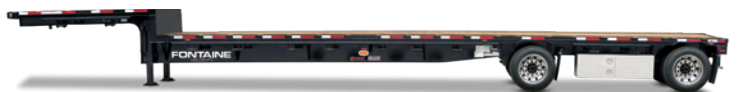
Velocity wide spread air ride dropdeck 48' or 53' configurations • Frame rating 80,000 lbs distributed
