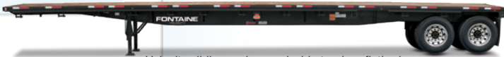
Velocity sliding spring or air ride tandem flatbed 45', 48' or 53' configurations • Frame rating 80,000 lbs distributed
