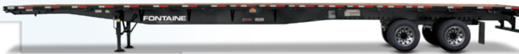
Velocity sliding spring tandem flatbed 48' configuration (setup for Canada) • Frame rating 80,000 lbs distributed
