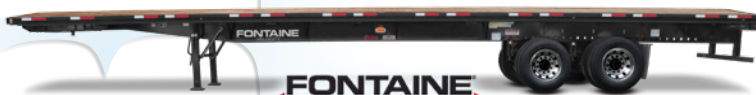
The Velocity SuperiorSlide™ air ride flatbed INDEPENDENT SLIDING AXLES for better load distribution and easier compliance 48' or 53' configurations • Frame rating 80,000 lbs distributed
