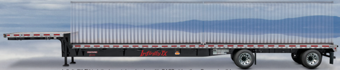
Infinity™ TX twistlock container hauler with RASR siderails • Rear axle slide
