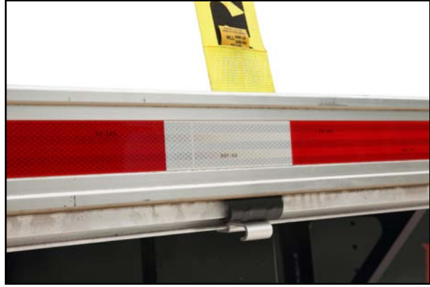
Figure 2: Strap hook inserted in side rail slot secured by sliding hook retainer WLL = 5400 lbs. (2449 kgs)
