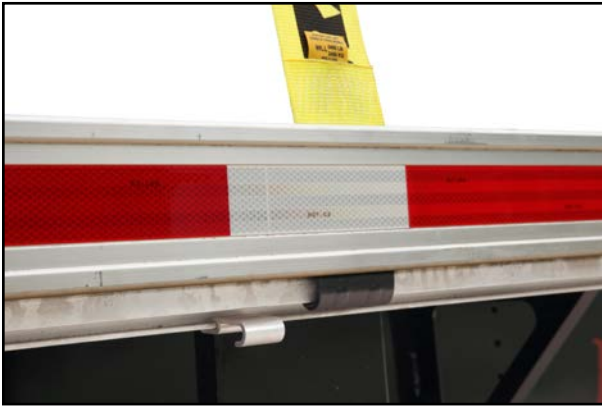
Figure 2: Strap hook inserted in side rail slot WLL = 5400 lbs. (2449 kgs)
