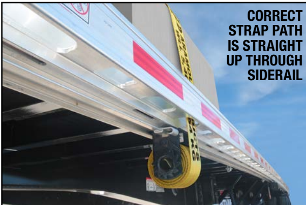
Figure 2: Strap hook inserted in side rail slot WLL = 5400 lbs. (2449 kgs)
