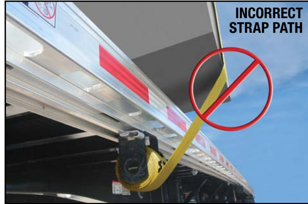
Figure 2: Strap hook inserted in side rail slot secured by sliding hook retainer WLL = 5400 lbs. (2449 kgs)
