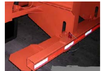
Figure B: Bumper tube positioned for trailer operation with no forklift.
