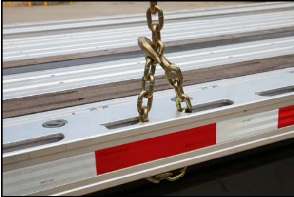
Figure 1: Chain securement through stake pocket and chain slot WLL = 5400 lbs. (2449 kgs)
