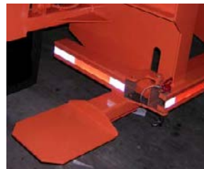
Figure A: Bumper tube positioned to allow forklift to be loaded.
