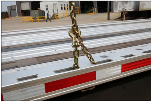
Figure 2: Chain securement through two chain slots WLL = 5400 lbs. (2449 kgs)
