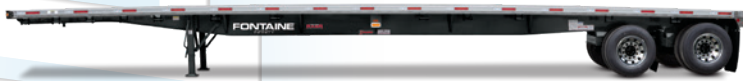
Infinity sliding spring or air ride tandem flatbed 45', 48' or 53' configurations • Frame rating 80,000 lbs distributed
