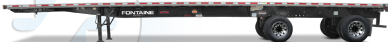
Infinity sliding axle air ride flatbed 48' front axle slide • 53' rear axle slide • Frame rating 80,000 lbs distributed
