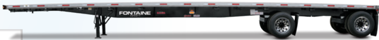
Infinity wide spread air ride flatbed 48' or 53' configurations • Frame rating 80,000 lbs distributed
