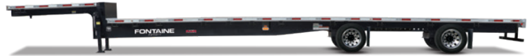
Infinity rear sliding axle air ride dropdeck 53' configuration • Frame rating 80,000 lbs distributed
