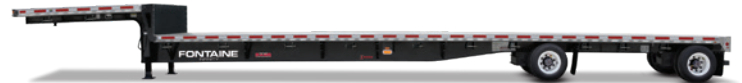
Infinity rear sliding axle air ride low height dropdeck 53' configuration • 36" loaded deck height • Frame rating 80,000 lbs distributed
