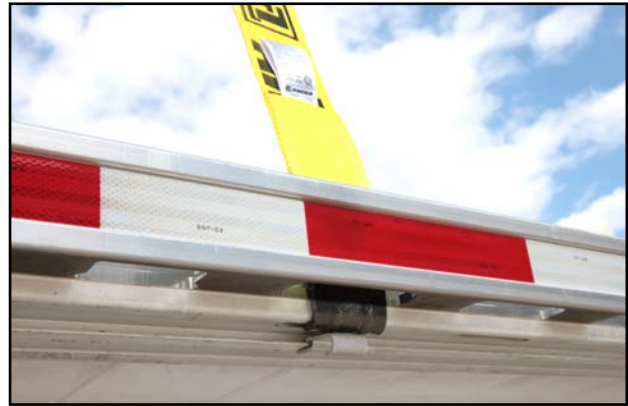
Figure 2: Strap Hook Secured in Side Rail Slot WLL = 5400 lbs. (2449 kgs)
