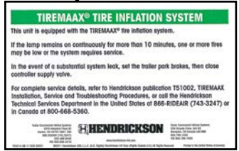
TireMaax Equipped Decal is only on Trailers with the option. Located on trailer front.
