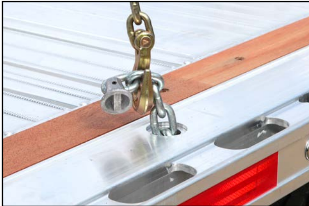
Figure 3: Chain Tiedown Security WLL = 5400 lbs. (2449 kgs)
